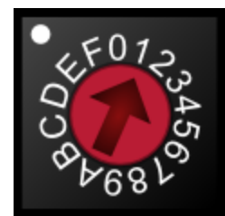
Figure 3 Address switch (SW3) with address 1 selected
