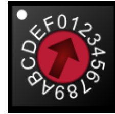
Figure 3 Address switch (SW1) with address 1 selected
